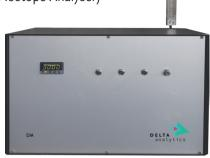
NDIR technology for measuring the isotope ratio of CO<sub>2</sub> in environmental air. Specifications:
